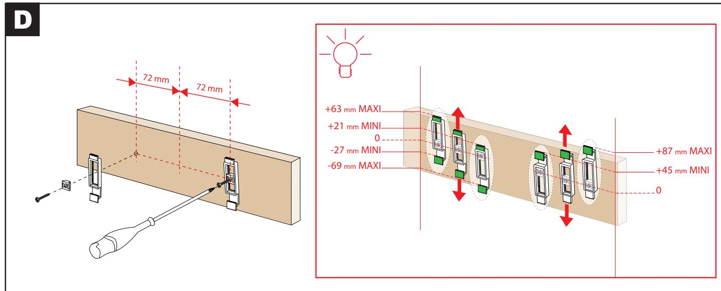
Screw the 2 cistern wall supports to the back of the unit.
