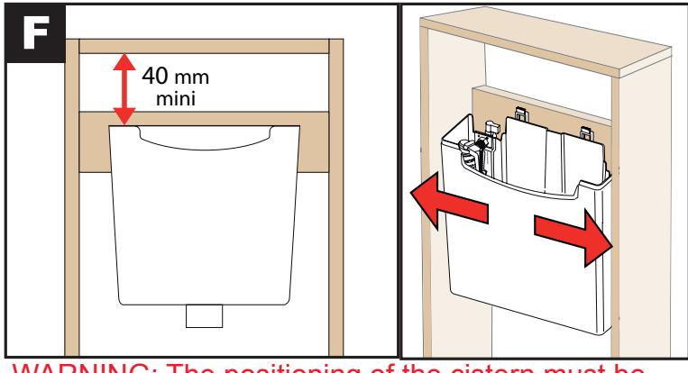
**WARNING:** The positioning of the cistern must be 40mm minimum from the underside of the furniture or worktop. Horizontal adjustment of the cistern is possible after installation on the brackets.
