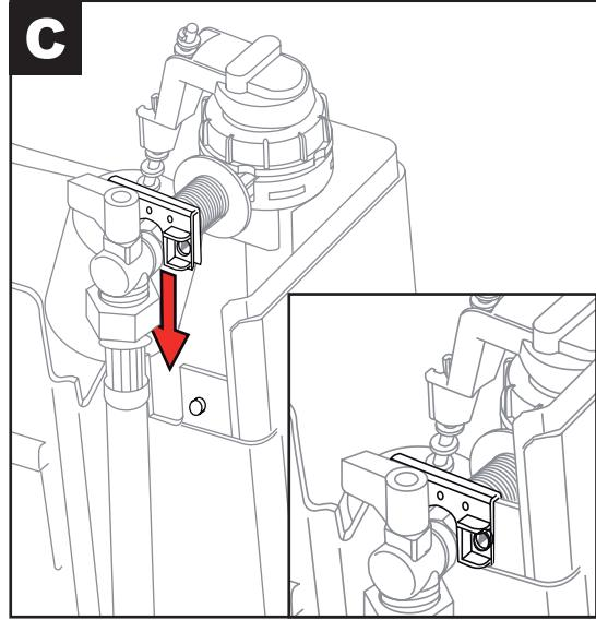
**NOTE:** Turn the TOPY float to the right if connection is on the left, or to the left if connection is on the right.
