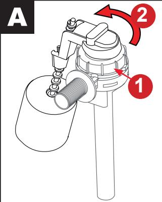
Unscrew the nut **1** of the Topy inlet valve. Rotate the head **2** of the inlet valve and screw the nut **1** back on.
