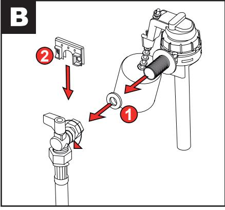
Fix the Topy inlet valve onto the isolation valve.
